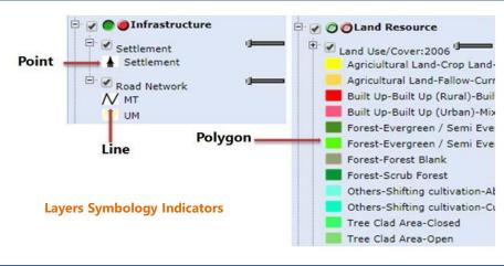
Symbology Indicators provide a visual indicator for the layer. In GIS, the appearance of the layer within the map is called the layer's symbology. In the Legend Window, polygons are indicated by a polygon, or square box, lines are indicated by a line, and points by a small dot. Raster images are indicated either by a camera icon or by a square box, depending on the type of image.
